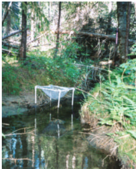
Leaf-litter trap in Dark Canyon Creek, used to monitor seasonal changes in leaf-litter input before and after prescribed fire. [photo by Leah Rogers]
