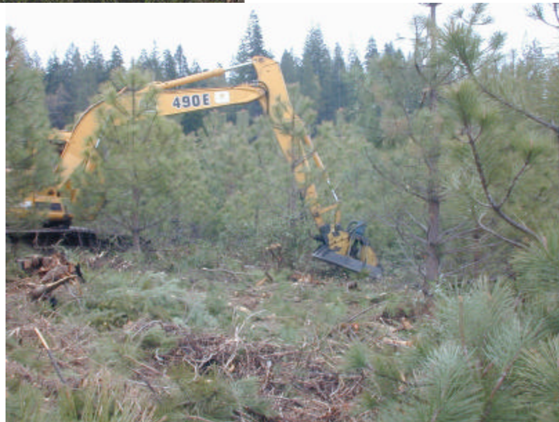
Right: A masticator efficiently pre- commercial thins an average of 3-4 acres per day.
