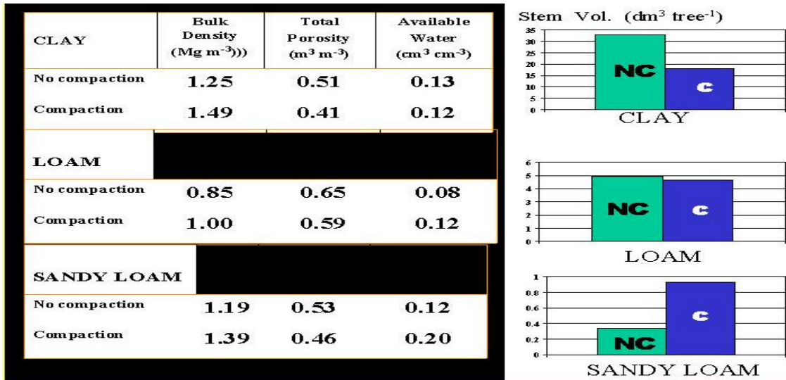
Figure 1. Effects of soil compaction (C) on soil physical properties, water availability, and tree growth for three contrasting soil textures. Soils are from Challenge (clay), Blodgett (loam) and Rogers (sandy loam) LTSP sites in California.
