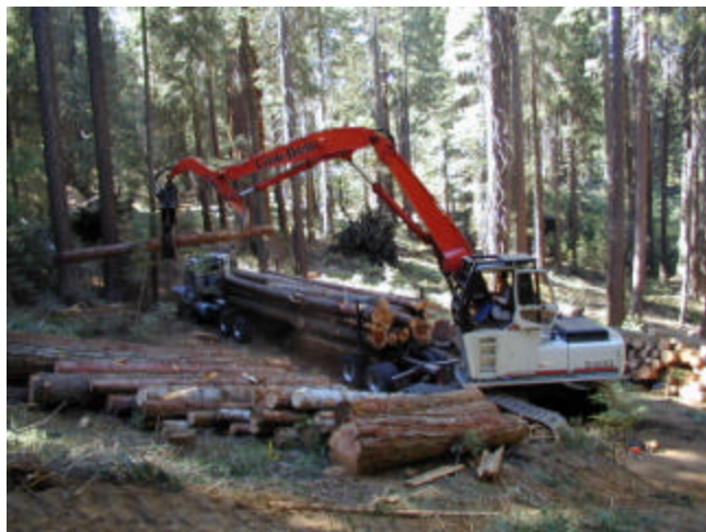
Right: HEEL BOOM LOADER STACKING LOGS IN A LANDING ON WHITAKER FOREST
